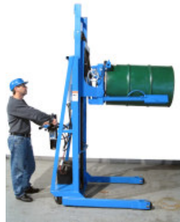
4. Release the clamp, then raise your drum to place it on a rack up to 8.5 feet high on a 4-tier rack.
